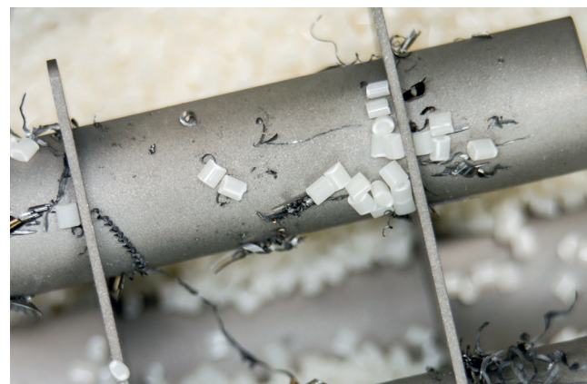
Smooth stainless steel cover for easy removal of particles
